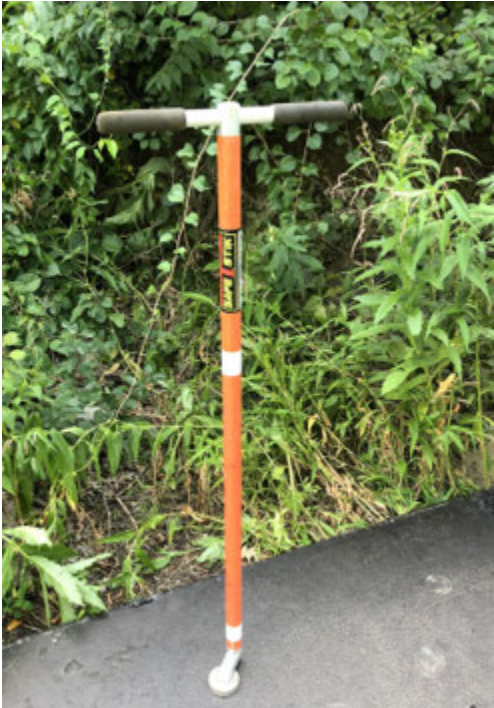
Figure B-11: Safe Stick for Guiding Steel Plates
