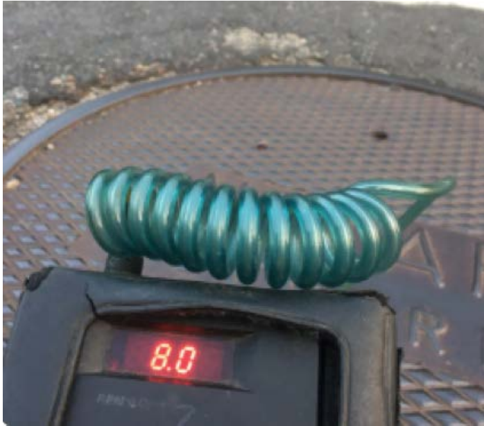
Figure 3. Recent example of a Grade 1 leak in a utility manhole in the westbound lane of Washington Street at Harrington Street, Newton, Massachusetts. Combustible gas in a confined space becomes hazardous at 4%; the concentration in this utility manhole was a sustained 8%.
